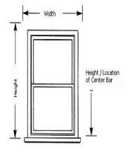
The Standard Window Size is  $(3' \times 5') 35'' \times 60''$  This worksheet is based on this standard  $3' \times 5'$  - most installed size window on homes and is usually located on all 4 sides and the 2nd story. Larger windows can be found on the front and back sides and are mostly on the 1st floor. Smaller windows are usually located on on the sides and around entry areas.
