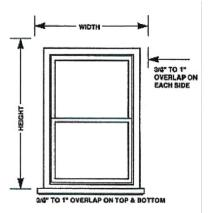
The Standard Window Size is (3'x5') 35"x60". This worksheet is based on this standard 3'x5' – most installed size window on homes and is usually located on all 4 sides and the 2<sup>nd</sup> story. Larger windows can be found on the front and back sides and are mostly on the 1<sup>st</sup> floor. Smaller windows are usually located on the sides and around entry areas.
